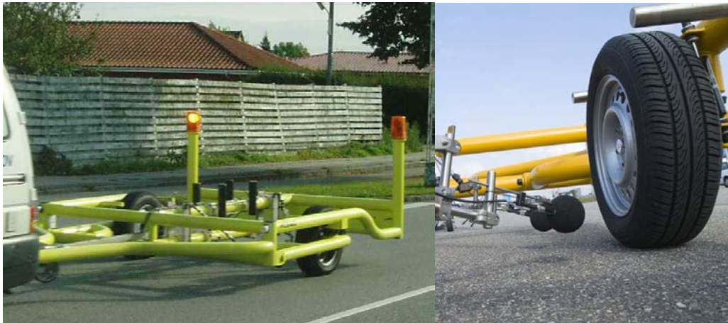
Figure 3: CPX noise measurement trailer (DRD)
