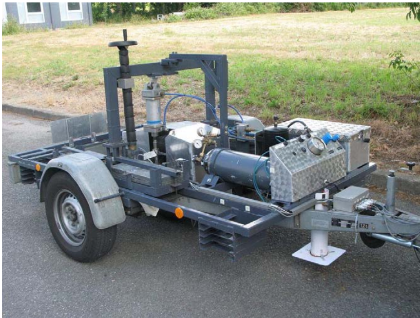
Figure 4: Rolling resistance measurement trailer (BAST)
